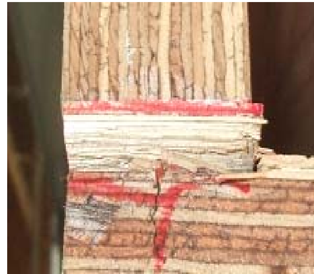
端部直交単板のrolling shear(右)
